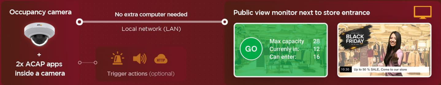
Compatible AXIS network camera (e.g. AXIS M3064-V / M3065-V etc.)
